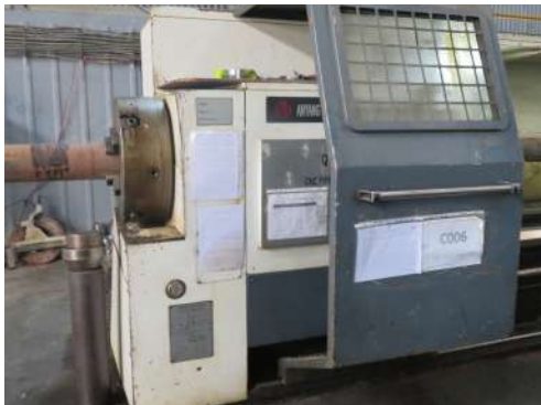
Turning CNC & Manual Fanuc Control MAX: Ø630 X5000
